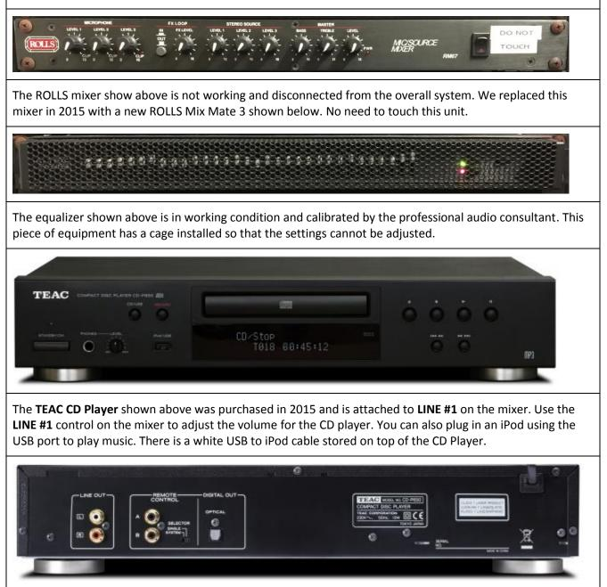
The picture above shows the backend of the CD player. The **LINE OUT** of the CD Player is attached to **LINE #1** on the Mixer.
